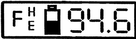
Figure 6 Low battery display
