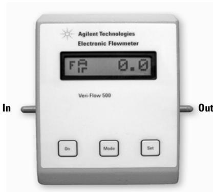
**Figure 1** Front view of gas connections
