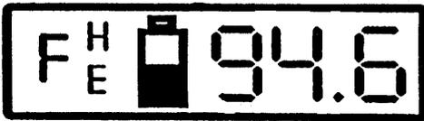
Figure 6 Low battery display
